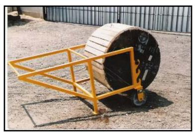
The yard trolley was designed to assist cable yard operations in speeding up the movement of drums to and from coiling machines. This is useful when forklifts are tied up or coiling machines are busy with long cut lengths as the drum can be rotated while on the yard trolley. This will be a manual operation but does give flexibility for short cut lengths. Sturdy wheels allow the trolley to be moved around in the yard as a one man operation.
